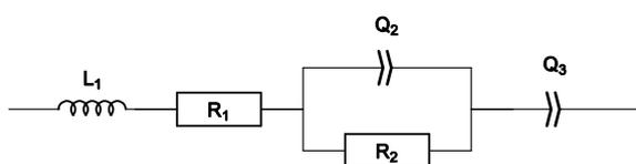
Figure 4: L1+R1+Q2/R2+Q3 equivalent electrical circuit.
