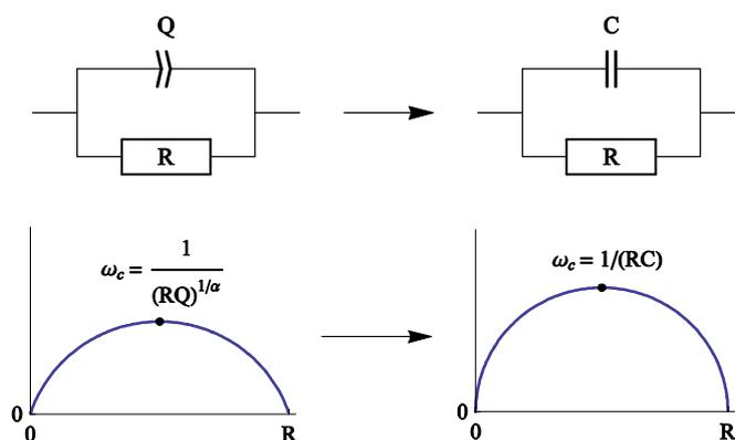
**Figure 1: Equivalent electrical circuit RQ and RC with the corresponding impedance diagram.**
