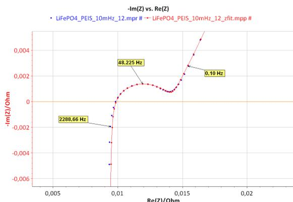
Figure 9: Nyquist impedance diagram (blue) and ZFit analysis (red) of a LiFePO4 battery with a  $L1+R1+Q2/(R2+Q3)$  equivalent circuit.
