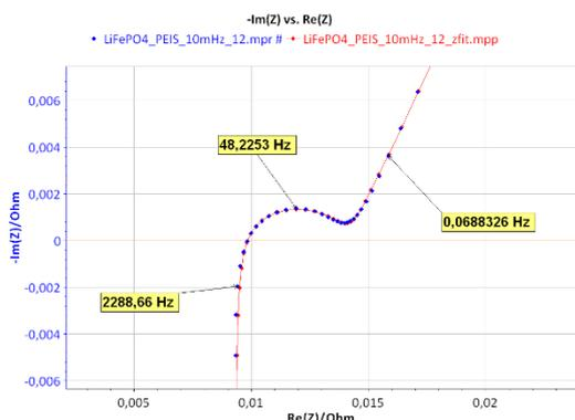
Figure 3: Nyquist impedance diagram (blue) and ZFit analysis (red) of a LiFePO<sub>4</sub> battery with a L1+R1+Q2/R2+Q3 equivalent circuit.
