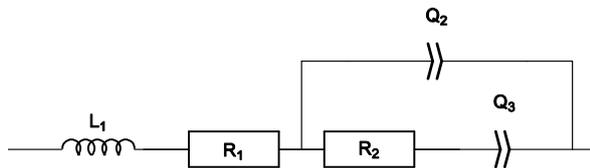
Figure 8:  $L1+R1+Q2/(R2+Q3)$  equivalent electrical circuit.
