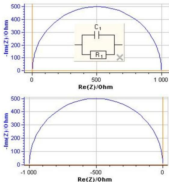
Figure 10: Nyquist diagrams for a RC parallel circuit.
