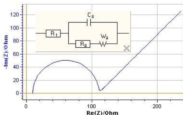
**Figure 4: Orthonormal Nyquist diagram for the Randles circuit.**
