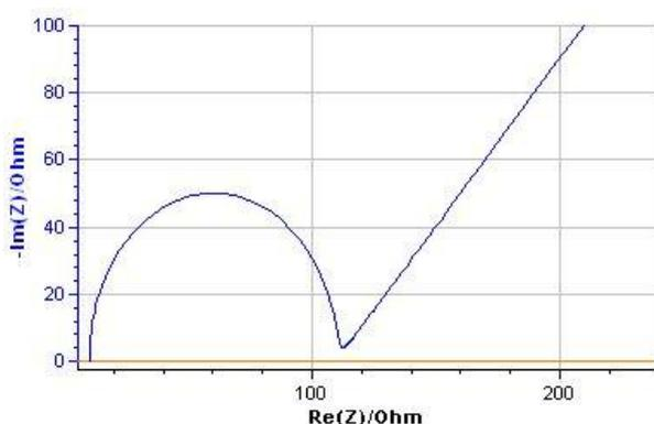
**Figure 5: Non orthonormal Nyquist diagram for the Randles circuit.**
