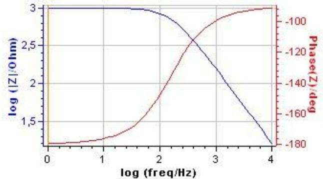
**Figure 8: Bode magnitude and phase plots for an RC parallel circuit.  $R = 10^3 \Omega$ ,  $C = 10^6$  F.**
