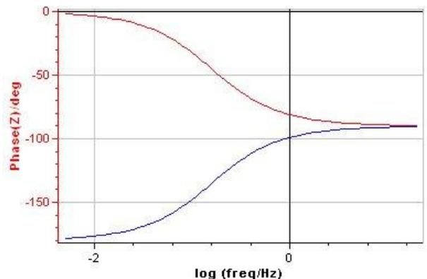
**Figure 9: Comparison of the impedance phase for  $R > 0$  (red) and  $R < 0$  (blue).**
