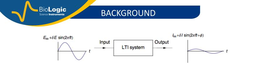
Current response has a the same frequency with an **amplitude**  $\delta I$  and **phase**  $\Phi$ Perturbation in potential, (it is also possible to perform the same in Galvano)
