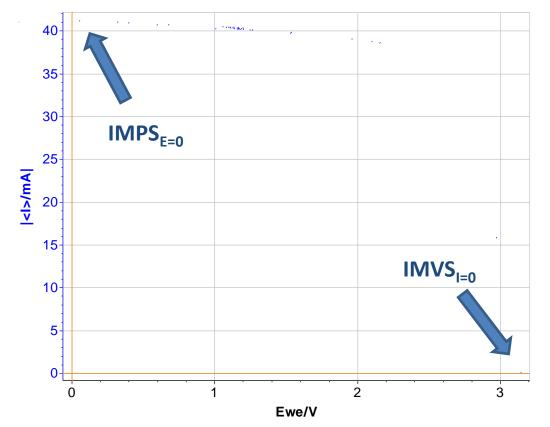
$IMVS = \mathcal{L}\Phi(t)/\mathcal{L}E(t)$  $IMPS = \mathcal{L}\Phi(t)/\mathcal{L}I(t)$
