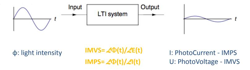
IMVS: Intensity Modulated photoVoltage Spectroscopy IMPS: Intensity Modulated Photocurrent Spectroscopy
