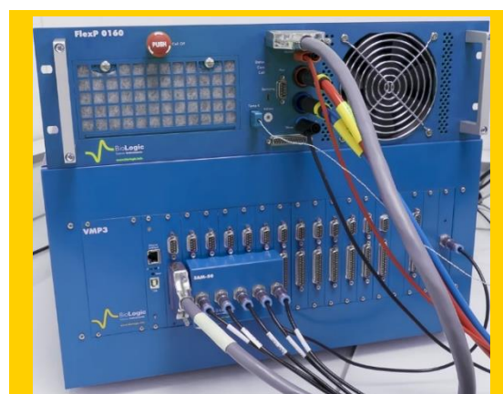
Figure 2 Hardware setup. VMP3 connected to the Current/voltage booster (FlexP 0160) on the top and SAM-50 plugged onto the VMP3 front panel.
