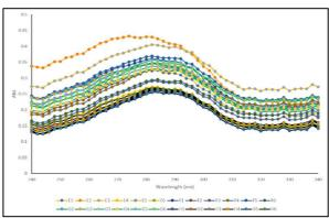
Fig. 4. Absorbance determinations of CSA by an unskilled technician. The Absorbance spectra of 200  $\mu l$  (+) CSA (Sigma) at 1 mg/ml in wells #A1-H12 of a solid silica bottom 96 well plate with black sidewalls (Porvair) from 240 - 340 nm were taken. Raw data were collected with no effort to minimize the noise or evaporation at a room temperature of 25°C. Representative data is shown in groupings of six and are color coded.
