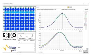
Fig. 3. Raw CD spectra of CSA. The CD spectra of 200  $\mu l$   $H_20$  & (+) CSA (Sigma) at 3 mg/ml in wells #A1-H12 of a solid fused silica 96 well plate with black sidewalls (Hellma) from 240 - 340 nm were taken. Raw data was collected with no effort to minimize the noise or evaporation at a room temperature of 25°C. Representative data from cells B1-B12 are shown.
