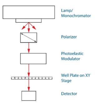
Block Diagram of the EKKO™ CD Microplate Reader
