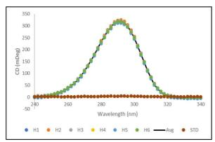
Fig. 5. Raw CD spectra of CSA from the final row of wells of an unskilled technician. The CD spectra of 200  $\mu$ I (+) CSA (Sigma) at 1 mg/ml in wells #H1-H6 of a solid silica bottom 96 well plate with black sidewalls (Porvair) from 240 - 340 nm were taken. Raw data were collected with no effort to minimize the noise or evaporation at a room temperature of 25°C. Wells H1-H6 are shown in addition to the mean and standard deviation of those six.
