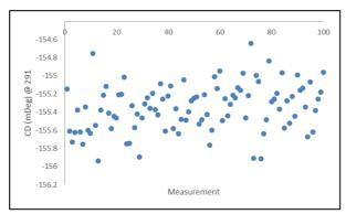
Fig. 1. Consecutive measurements in in wells A10 & F2 of (-) CSA as a function of measurement. Successive measurements of 200 µl of (-) CSA (Sigma) at 1 mg/ml in wells #A10 & #F2 of a solid fused silica 96 well plate (Hellma) taken at 291 nm. Data was collected with no effort to minimize evaporation (samples were not protected with an optically clear cover) or reduce the noise (data were collected with the shortest integration times possible) at a room temperature of 25°C.
