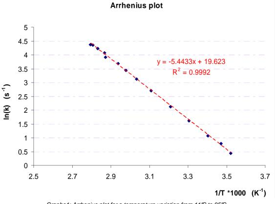
Graphe1: Arrhenius plot for a temperature variation from 11°C to 85°C
