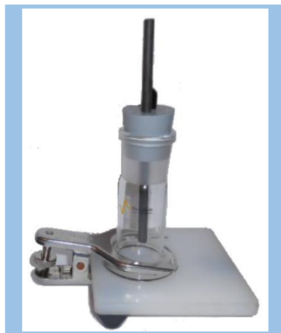
Figure 1 : Coating cell with a carbon rod counter electrode and an Ag/AgCl reference electrode.
